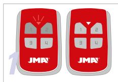
Press buttons 1 and 2 of the remote control copy simultaneously until the led flashes red. Release both buttons and wait for led red to turn off.
