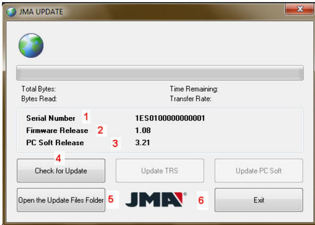
Sections (1), (2) and (3) respectively display the TRS EVO's manufacturer serial number, its current firmware version and the version of the PC software installed on the computer.
