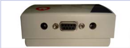
Picture 2 . Back side of the TPX CLONER with the DC connectors and Serial Comm.
