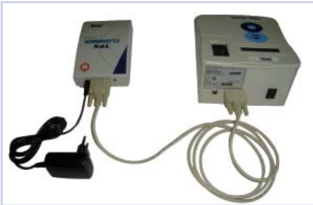
Picture 3. Second of the three steps to connect the TPX CLONER to the TRS5000.
