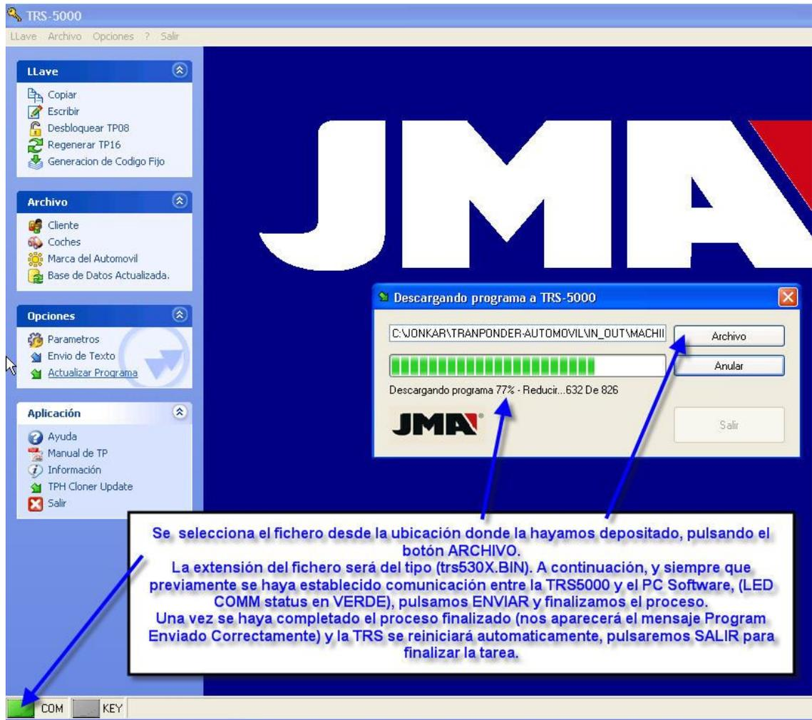
NOTE: The COM status LED must be green, which indicates there is communication between the PC-TRS5000.
