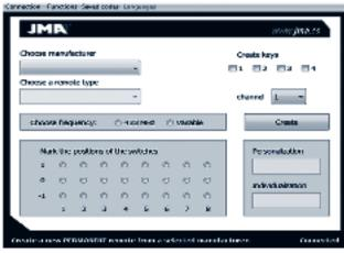
Select the manufacturer, the type of remote you wish to generate, the frequency, desired switch positions, the channel and the SR remote buttons on which this remote is to be generated.
