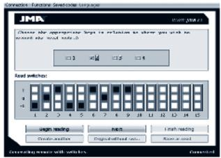
Once all of the buttons have been selected, when you press 'Next' the application will show the position in which you have to place the switches on the original remote and the position in which you have to place the switches on the duplicate remote, where relevant. Duplication is now finished.
