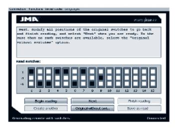
Once you have modified all the positions, press 'Next'. Then repeat the same readings of the original remote, but this time with the switches changed. Once the same number of readings have been repeated, press 'Next' and the following message will appear indicating that the readings have been carried out.
