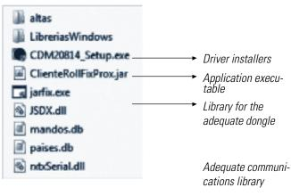
First execute the driver installers. The following screen will appear indicating: "Installing driver..." and "FTDI CDM Driver Installation process completed" when the driver has been installed.
