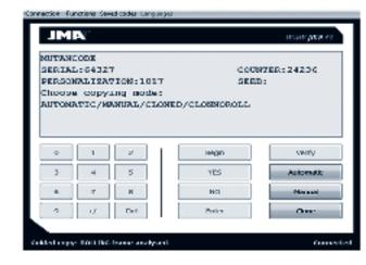
As when making a Guided duplicate, when the remote analysed is a fixed code remote it asks you to press 'Enter' to read the complete code from the start.
