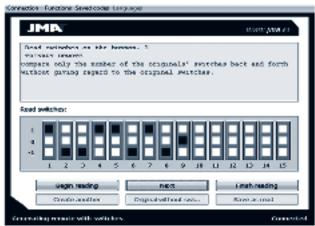
Then, if there are more buttons for recording information than the original remote, press 'Next' and the application will ask you to press the corresponding button. If all of the original remote's buttons have been read, press 'Finish readings'.
